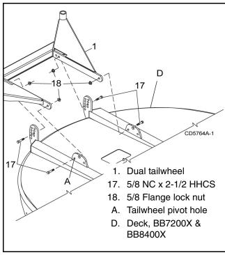
Figure 35. Dual Tailwheel Installation
